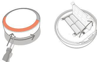
**EN** Remove the wall-mounted siren using a screwdriver (press and turn the siren). Open the battery cover in the direction indicated by the arrow and replace the batteries. / **FR** Remplacement des piles.
